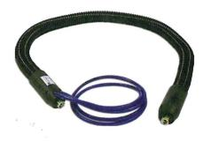
The HDM 60 (max. 60°C) and HDM 62 (max. 200°C) heat transfer hoses are built similar to electrically heated hoses. In these hoses the heating conductor is replaced by a wound hose in which the heat carrier flows. Heat transfer
